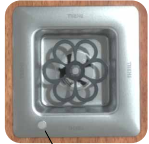
Battery recharge connector
